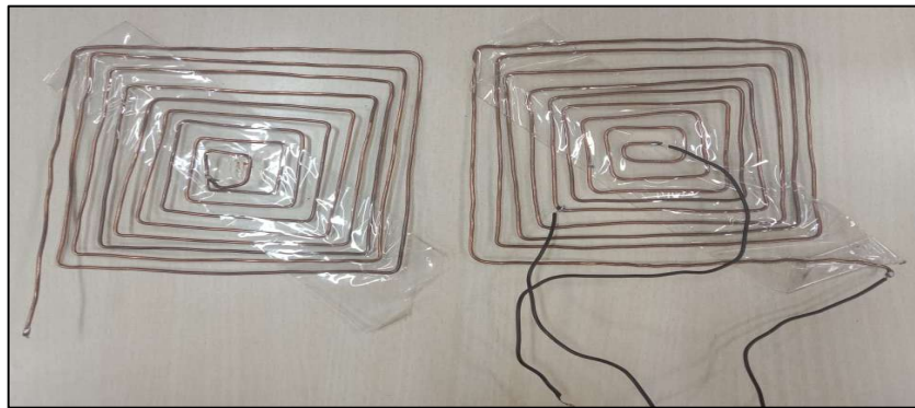
Figure 5. Square spiral coil of 10 turns with thickness of 2mm with 1mm gap.
